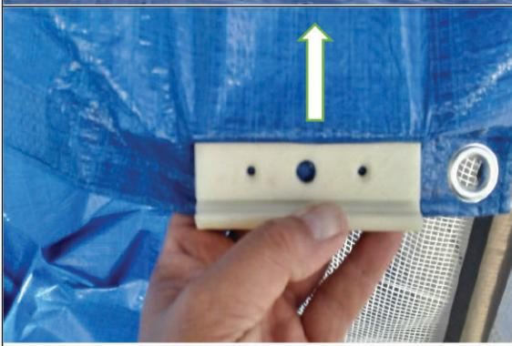
**NOTE:** You must use a hand screwdriver ONLY to snugly secure the screws in place as the Clip and Vice can easily crack if the screw head rotates too tightly. THIS WILL VOID RETURNS.
